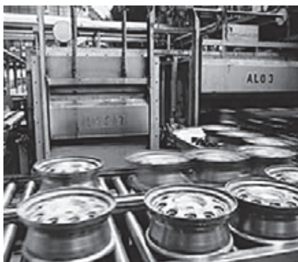
Aluminium industry: curing oven for wheel rims
