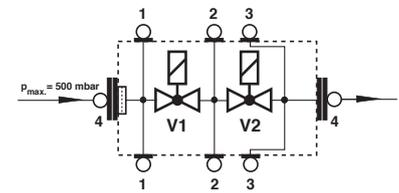
The seal plugs **1,2,3** can also be replaced by a G 1/8 instrument gland as per DIN ISO 228
