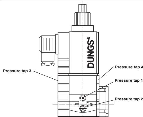
Pressure taps for 1, 2 and 4 are installed depending on the SV model.
