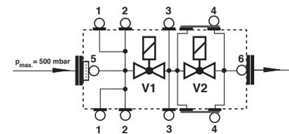
The seal plugs **1,2,3,4** can also be replaced by a G 1/8 instrument gland as per DIN ISO 228
