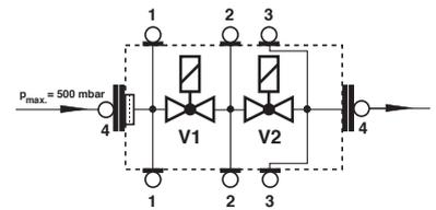
The seal plugs **1,2,4** can also be replaced by an instrument gland
