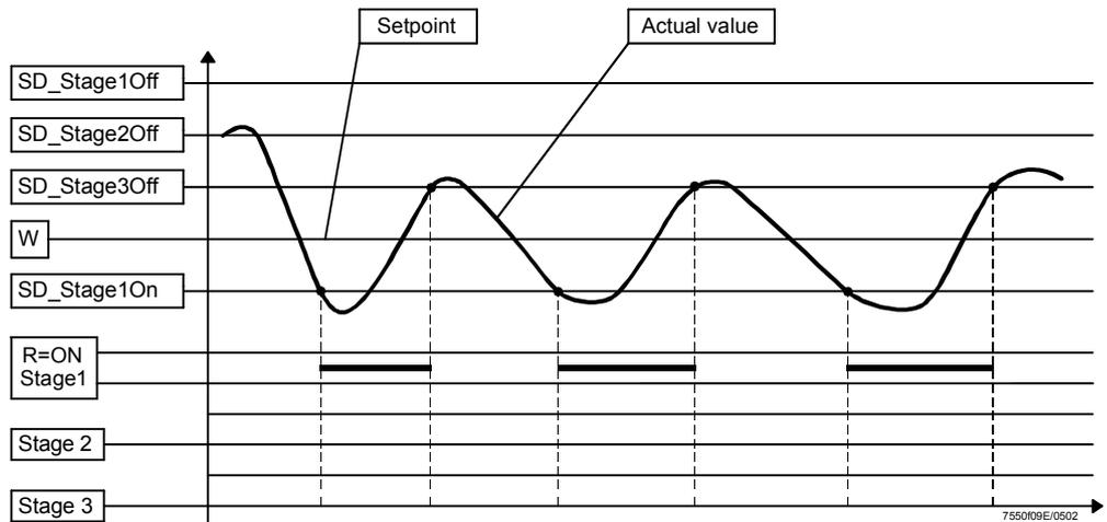
Example 2: Reaction thresholds Q2 and Q3 for switching on stages 2 and 3 are exceeded and the stages will be switched on. In that case, stage 1 will be switched off when threshold  $W+SD\_Stage1Off$  is reached.
