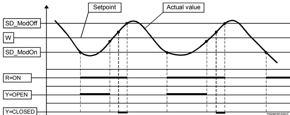
Example 2: The load is greater than the amount of heat produced by the burner under part load conditions, thus enabling correct modulating operation.
