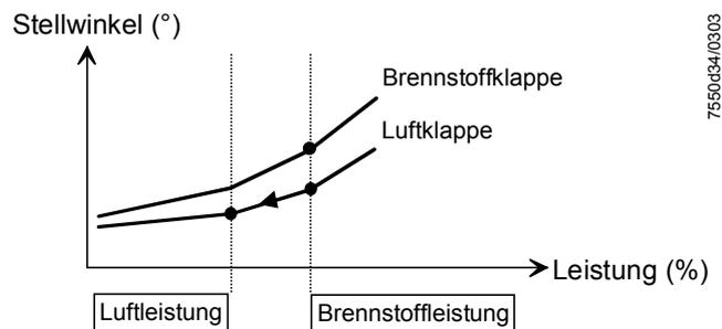
Due to the air rate reduction, the O<sub>2</sub> trim controller reduces the amount of air. For that purpose, the air-influencing actuators will travel to a smaller load (air rate) on the ratio curve. On the ratio curve, fuel rate and air rate are the same.
