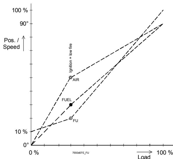
Change of load / position resulting from an automatically entered point
