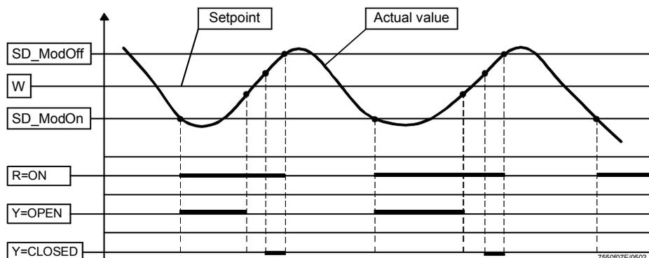
**Cold start thermal shock protection (CSTP)**
