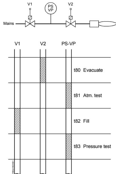
With gas valve proving, first the gas valve on the burner side is opened to bring the test space to atmospheric pressure.
