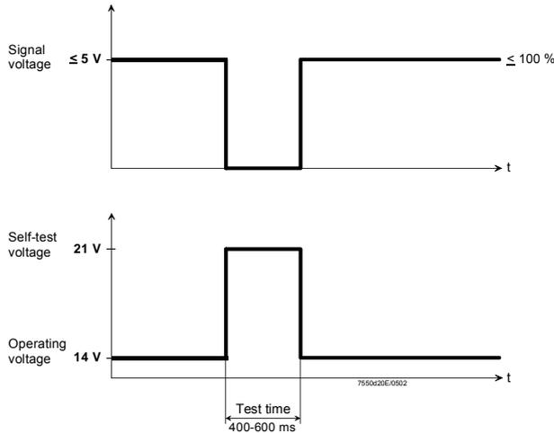
The self-test function of the QRI... is triggered by increasing the supply voltage to the level of self-test voltage.
