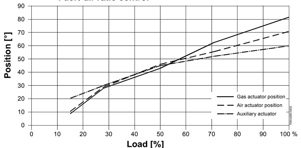
Changing an existing curve    The curvepoints can be changed during burner off periods (Phase 12) or during burner operation (Phase 60).
