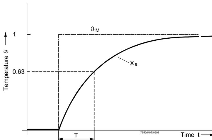
Instant temperature change of test medium to determine the time constant
